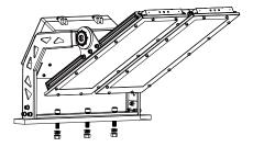
1. Put on the screws, flat washers, spring washers and nuts.
